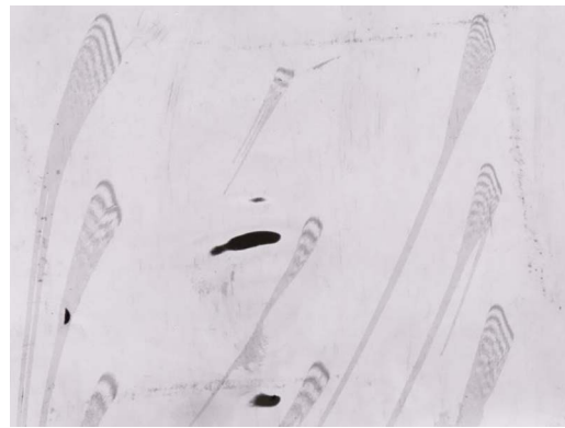
Fig. 4 Fringe patterns due to light interference from an oil patch thinned due to shear
